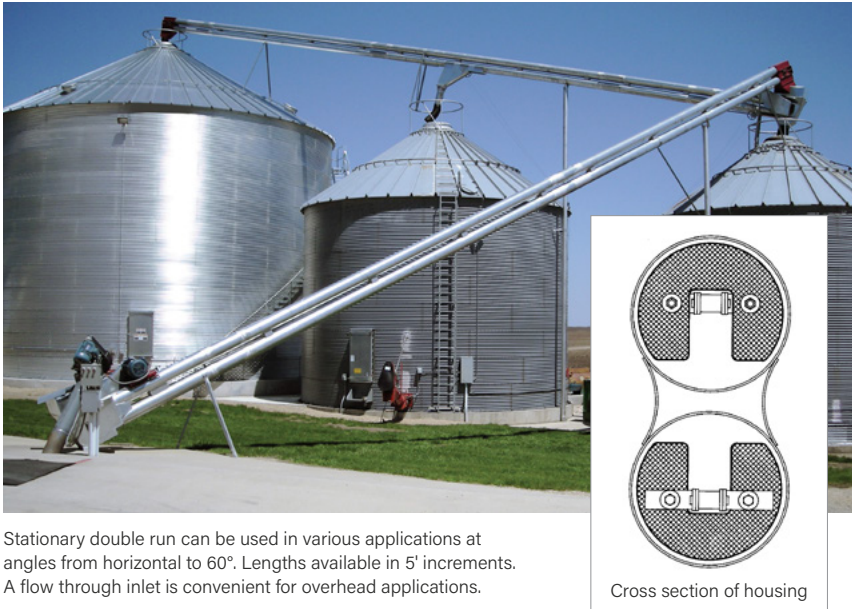
Stationary double run filling a dryer and unloading dryer to multiple bins.
