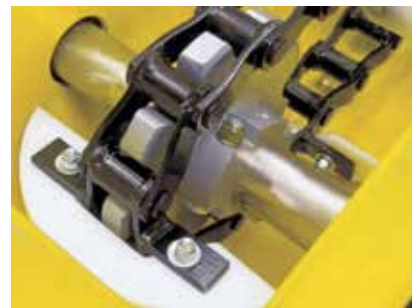
Flame hardened split sprocket for easy replacement
