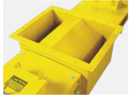
Bypass feed inlet allows feed to flow around return flight and travel directly to bottom run without damage to material
