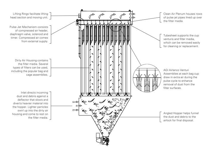
AGI Airlanco Pulse Jet Filters come in a variety of shapes, sizes, and filter bag layouts to fit a broad range of applications, but the cleaning cycle remains the same throughout the line of products.
