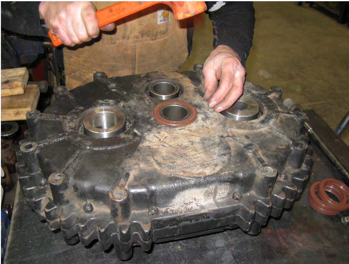
Figure 23. Installing Seals on Rear Casing Half
