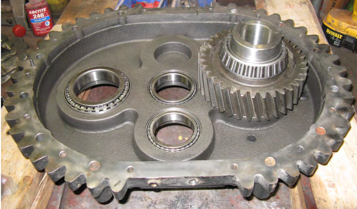
Figure 15. Installing the Bottom Shaft and Gear
