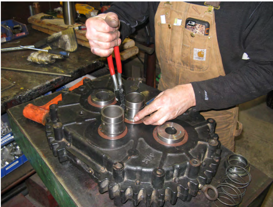
Figure 25. Installing Snap Rings
