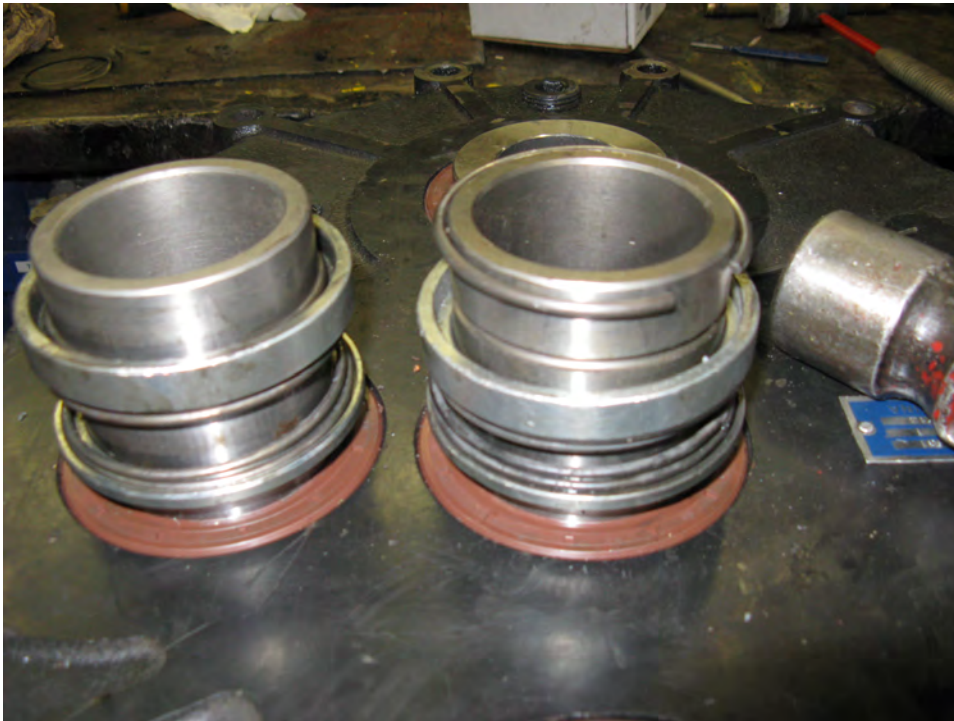
Figure 30. Installing Retaining Ring on Input Shaft
