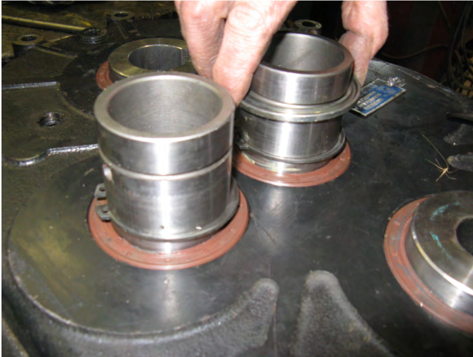
Figure 26. Installing Spring Base Rings
