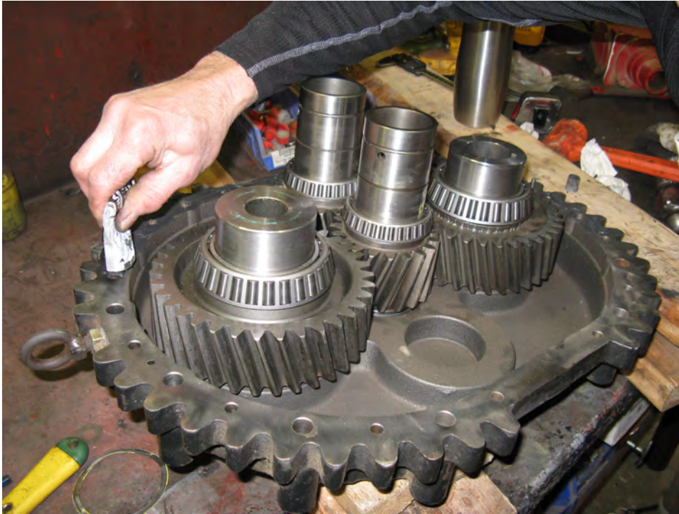
Figure 21. Applying Gasket-Maker to Front Casing Half
