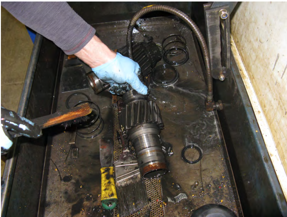
Figure 11. Cleaning Gearbox Components
