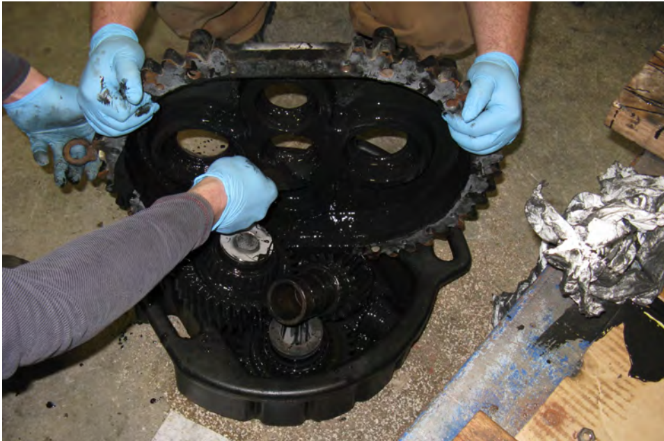
Figure 10. Dump Gearbox Components into Oil Pan
