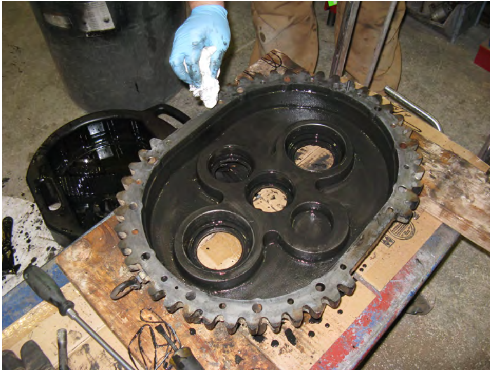
Figure 12. Cleaning Casing Halves
