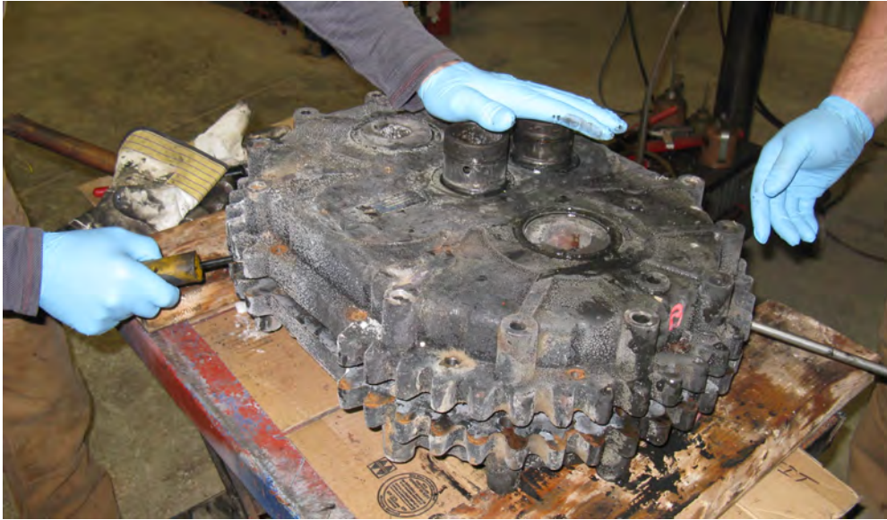
Figure 9. Front Casing Half Removed
