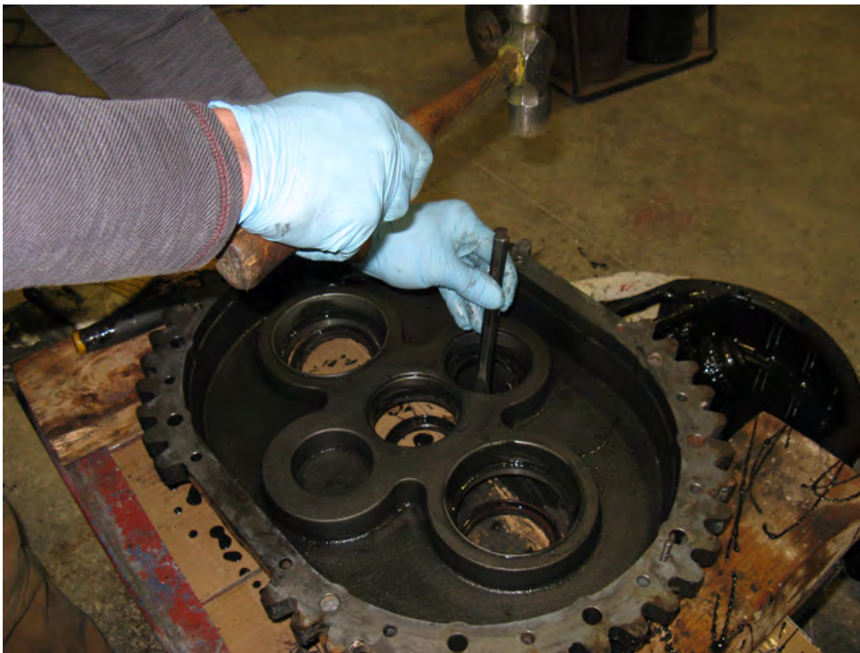
Figure 13. Removing Old Seals
