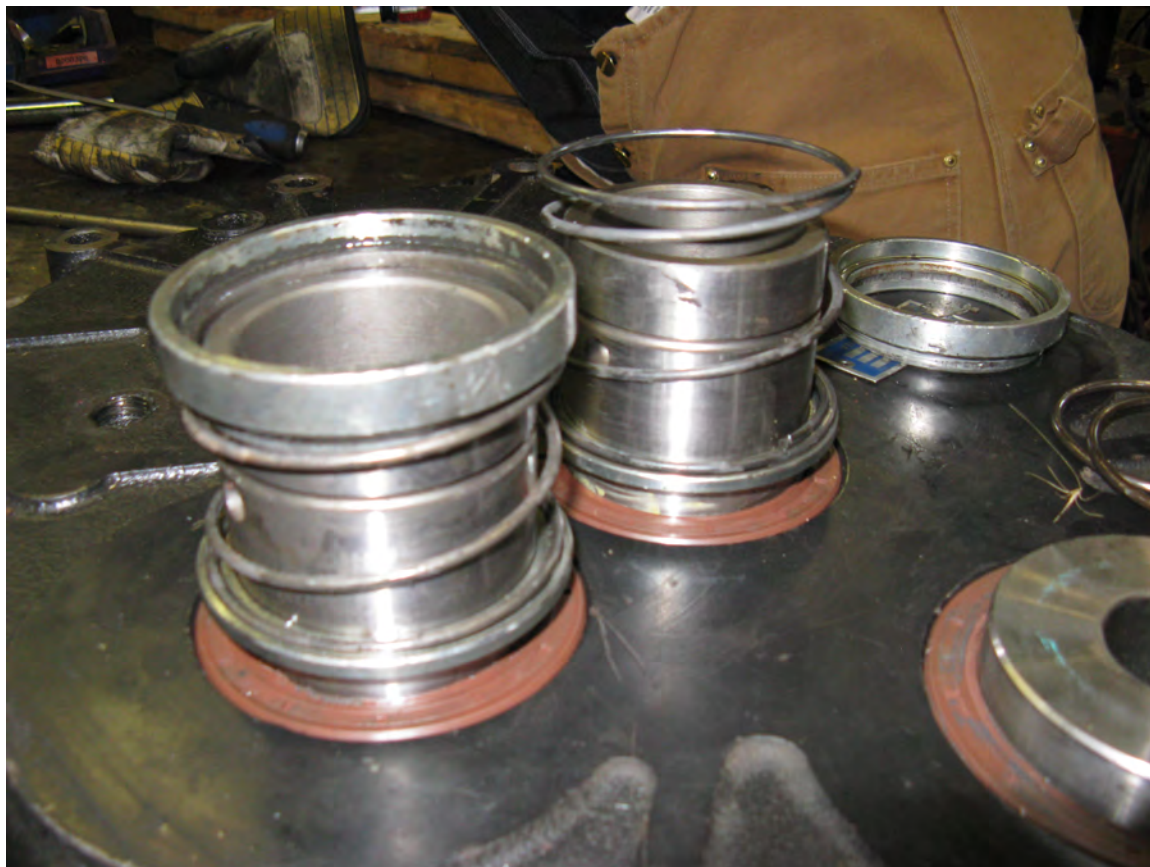
Figure 28. Installing Spring Top Rings
