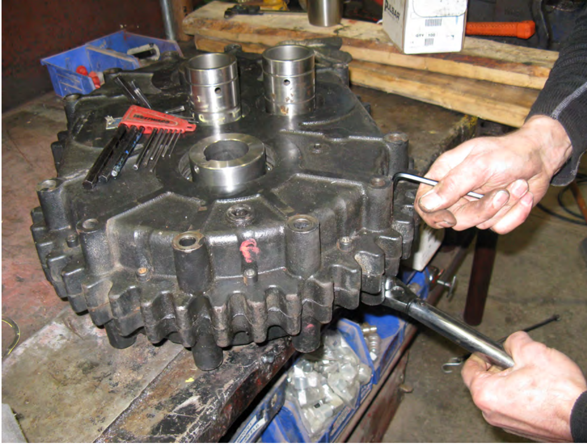
Figure 22. Fastening the Casing Halves Together
