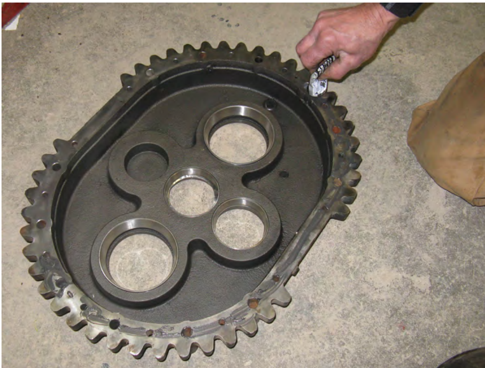
Figure 21. Applying Gasket-Maker to Front Casing Half
