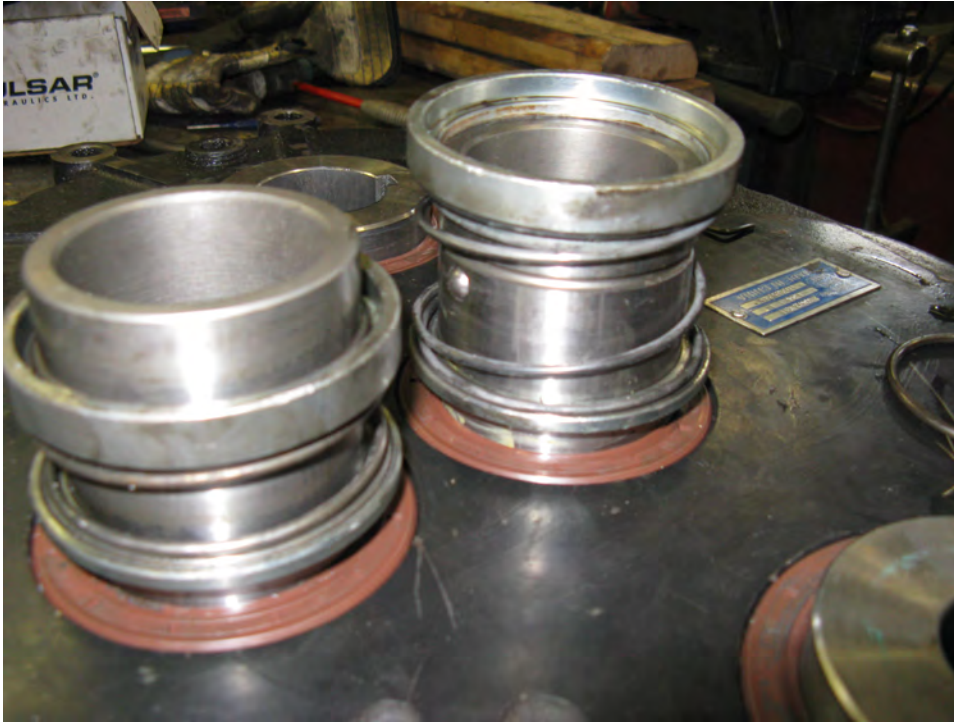
Figure 30. Installing Retaining Ring on Input Shaft
