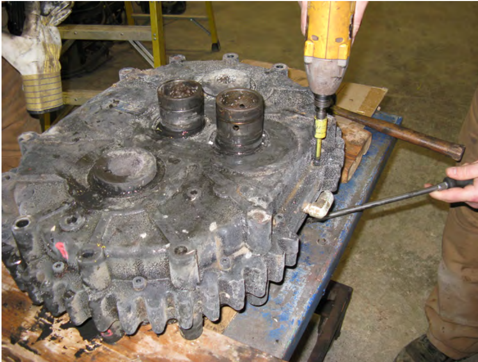
Figure 7. Removing Socket Head Screws
