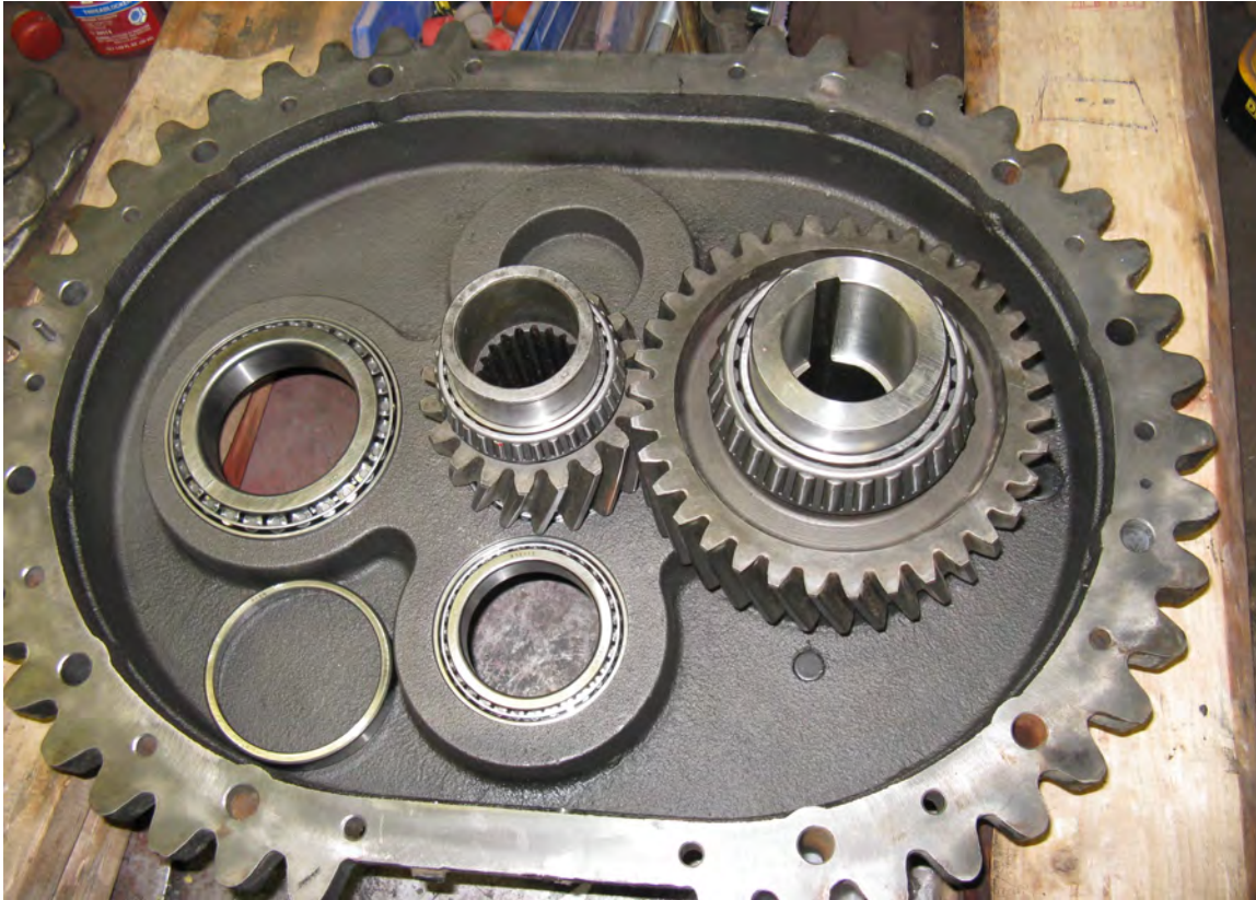
Figure 16. Installing the Input Shaft and Gear
