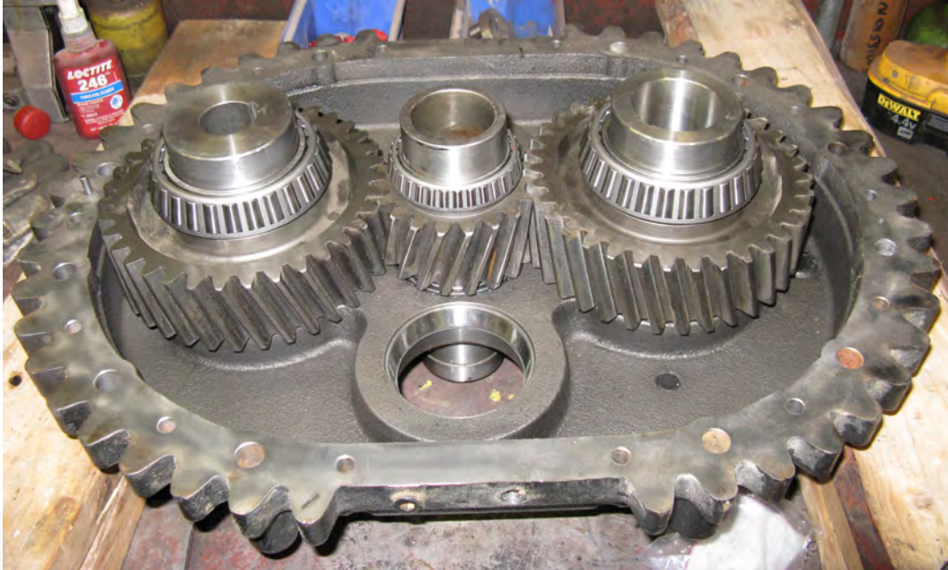
Figure 17. Installing the Top Shaft and Gear
