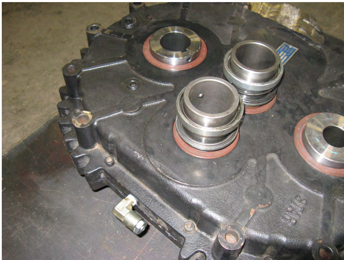
Figure 33. Checking Breather Vent Orientation
