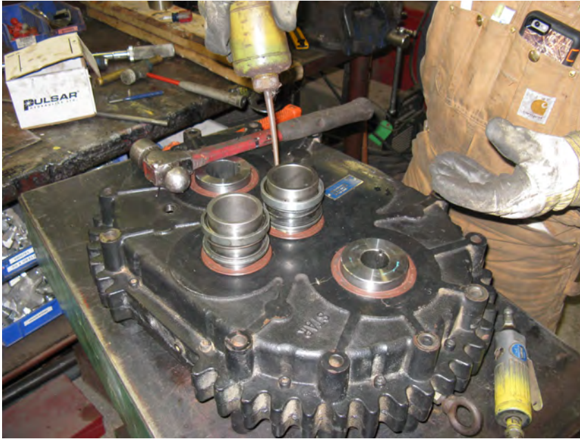
Figure 31. Lubricate Spring Components
