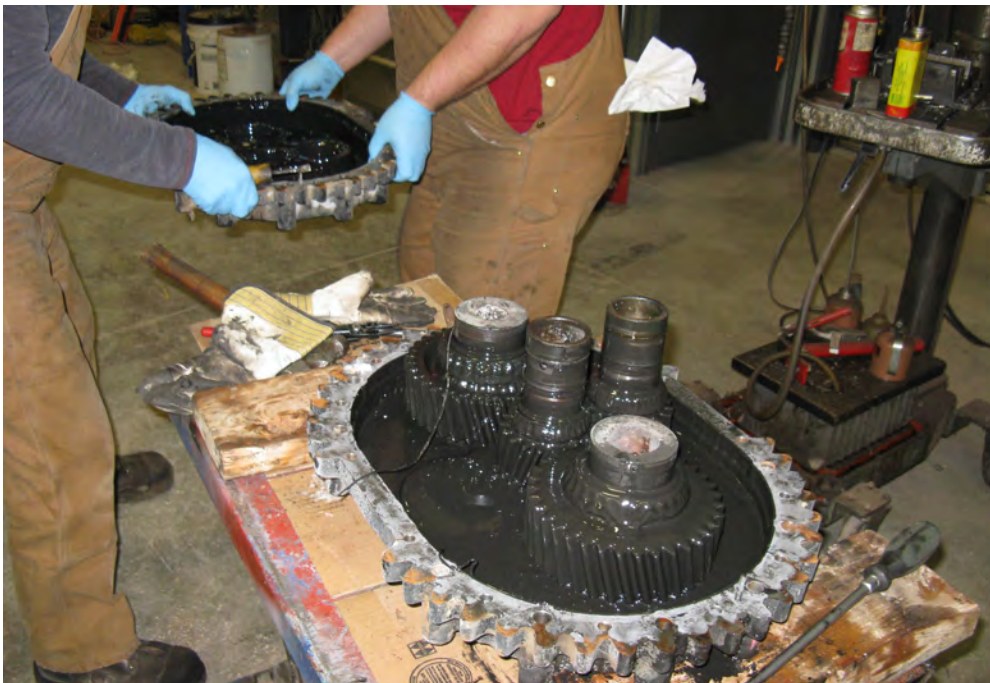
Figure 9. Front Casing Half Removed
