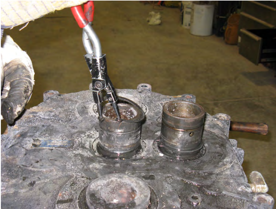
Figure 5. Removing Snap Rings
