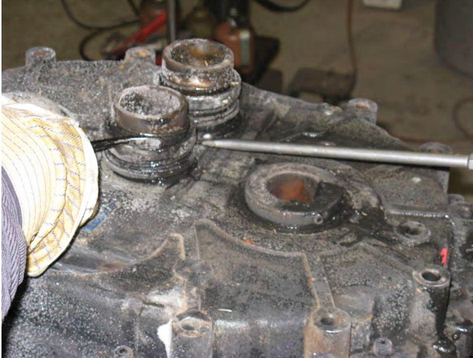
Figure 3. Removing Retaining Rings
