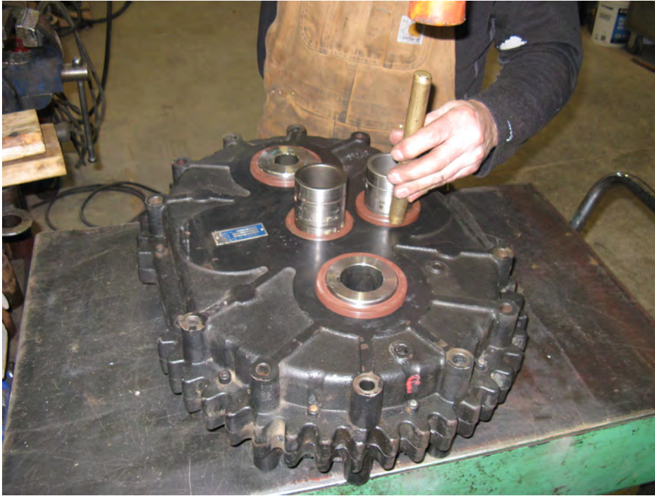
Figure 24. Installing Seals on Front Casing Half
