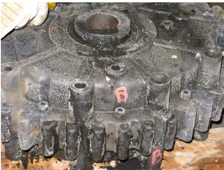
Figure 2. Mark Both Casing Halves
