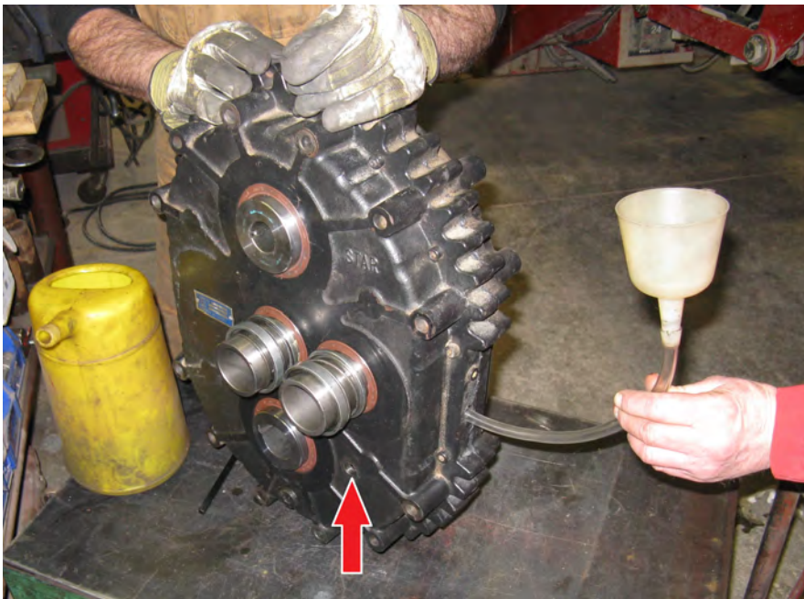
Figure 32. Fill Gearbox with Oil
