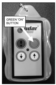
**Figure 4.2 Remote Transmitter**
