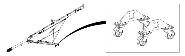
The caster kit attaches to the existing wheel hubs provided with the auger. The caster kit was designed to fit 4–bolt hubs.
