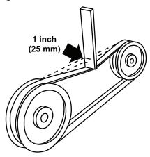
2. Tighten or loosen the drive belts (or idler pulley when equipped) to achieve the proper tension.
