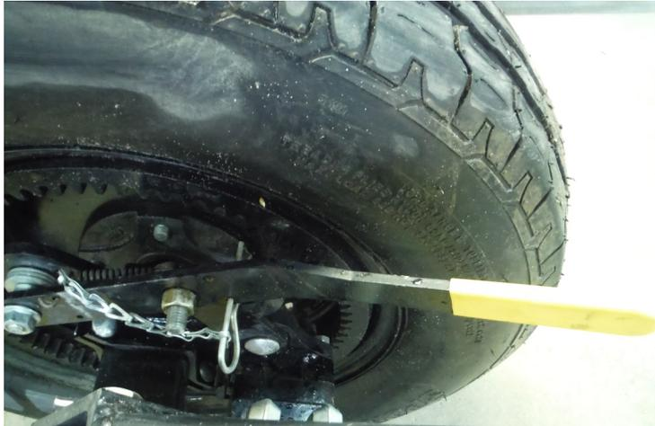
4. For transportation on public roadways, secure the v-frame to the auger frame to prevent it from accidentally slipping. Loop the snap link through the v-frame hook and attach it to the chain so there is as little slack as possible (Figure 4.3).
