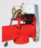
Upper drive has heavy-duty flangette ball bearing and adjustable motor mount with double "B" belts and pulley (triple belts on 13" models).
