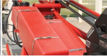
High capacity hydraulic pump and frame mounted oil reservoir.
