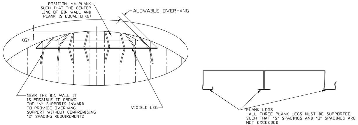
3. Position the second plank adjacent to the first and snap into place by applying downward pressure on the mating seam.
