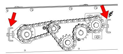
5. Tighten the chain tension roller idler bolt to 120ft-lb using a torque wrench.
