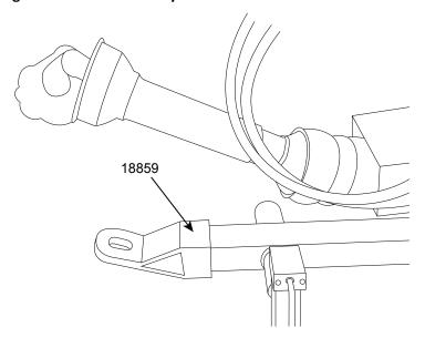
Figure 4. Auger Tube and Hopper Safety Decals
