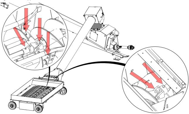
Figure 26. Upper Flighting Bearing Grease Point
