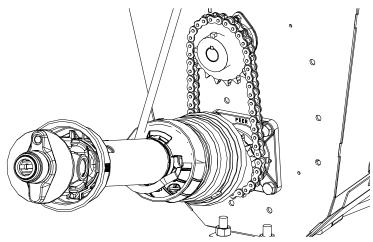
4. Tighten or loosen the adjustment nut on the side to set the chain slack for the hopper.
