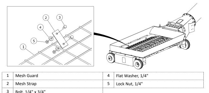
MARNING Install hopper mesh prior to operation of the auger.
