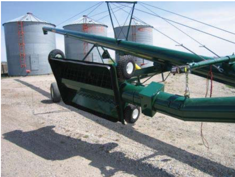
Figure 18. Hopper Rotated for Clean Out
