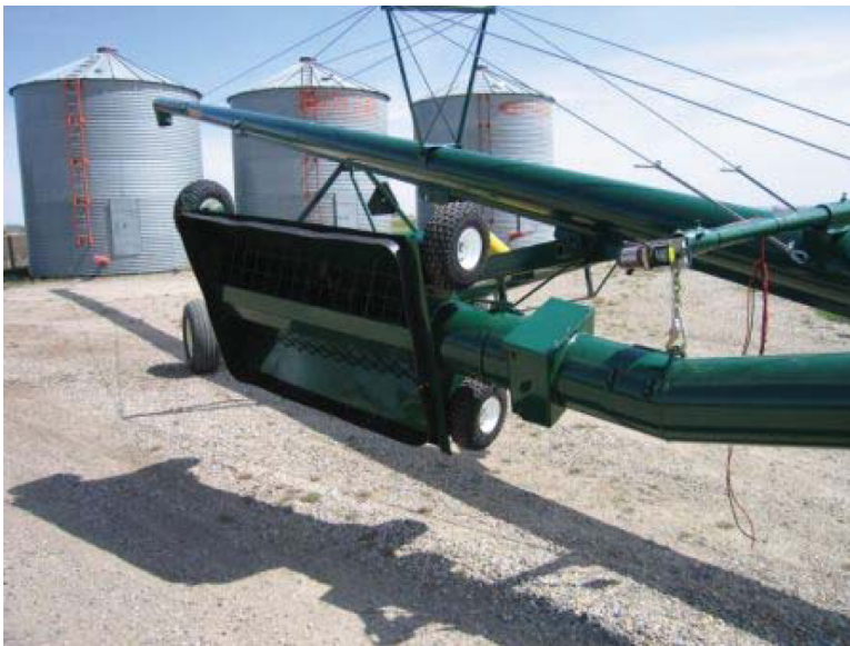
Figure 19. Swing-Away Hopper Storage Position
