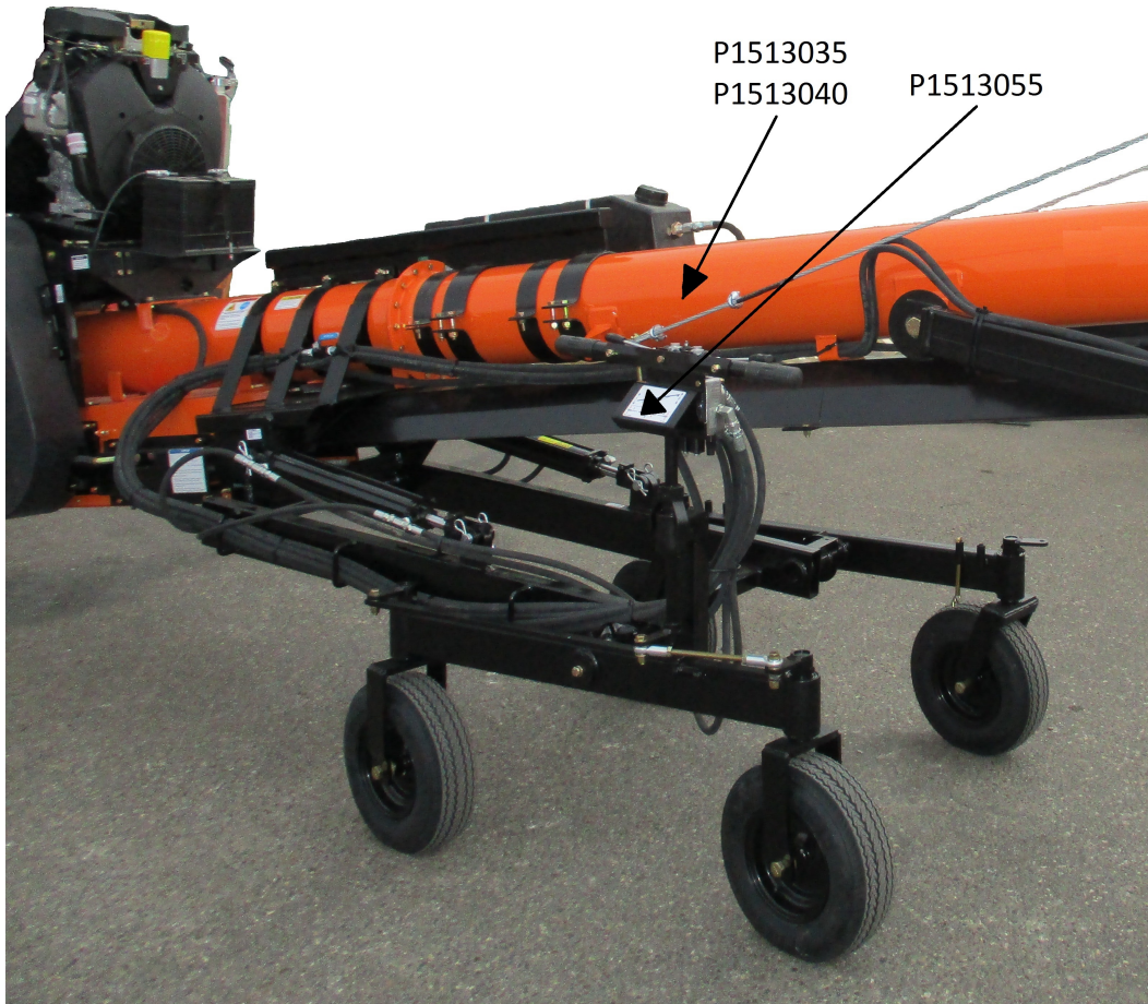
Figure 9. Wheel Move Kit for S-Drive Standard Conveyor (1500-Series) — Decal Locations
