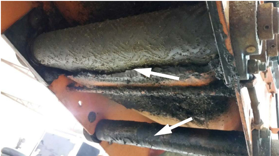
Figure 19. Fertilizer Buildup at Hopper Transition
