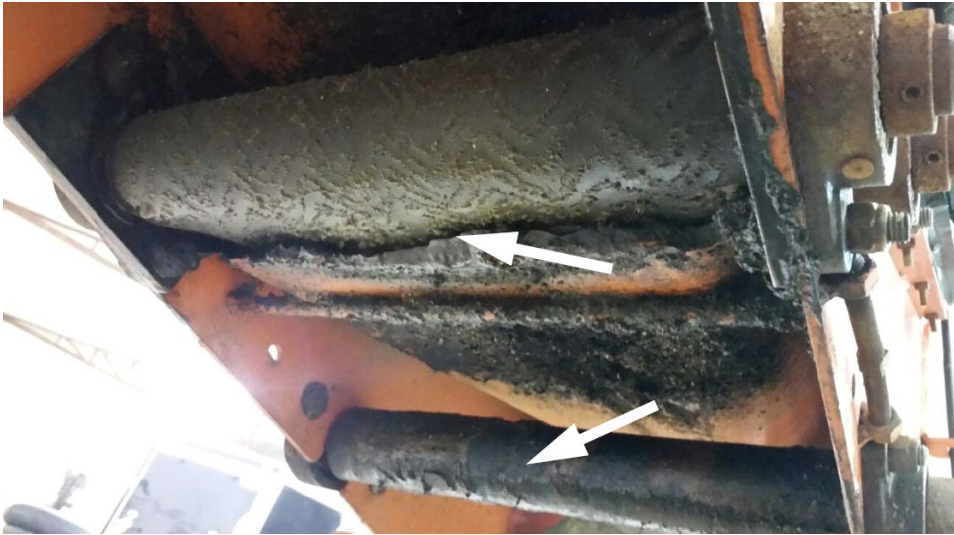
Figure 20. Fertilizer Buildup at Hopper Transition
