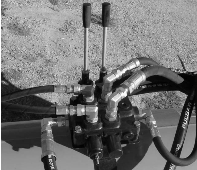
Figure 15. Power Swing Control Valve
