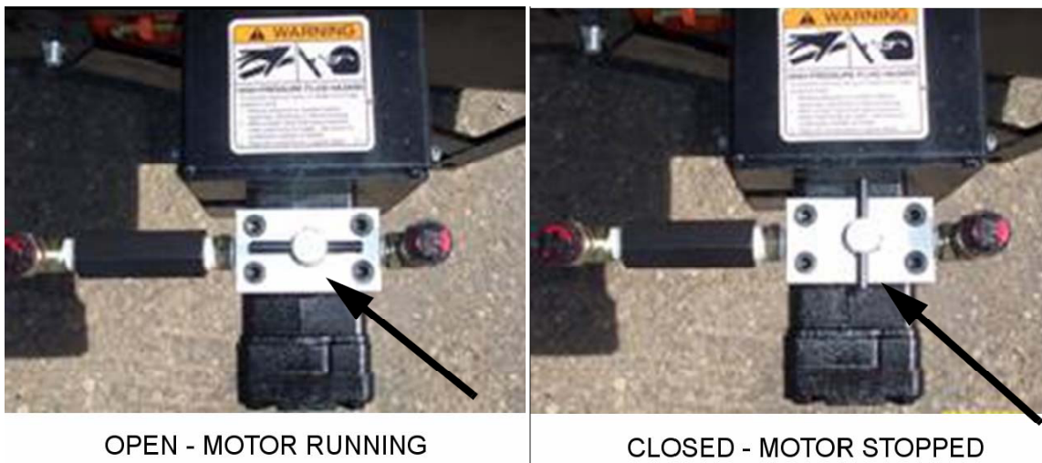
Figure 21. Hydraulic Drive Valve
