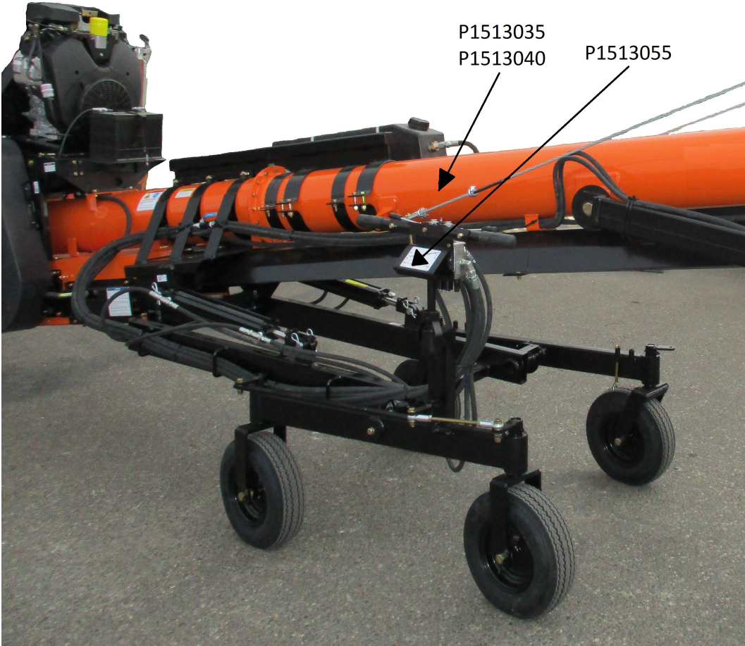
Figure 9. Wheel Move Kit (1800 and 2400 Series) — Decal Locations
