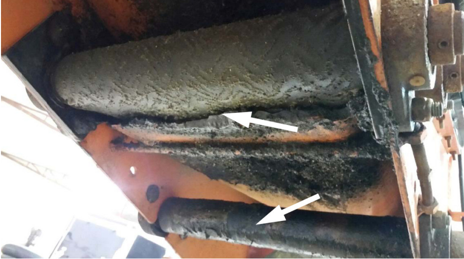
Figure 20. Fertilizer Buildup at Hopper Transition
