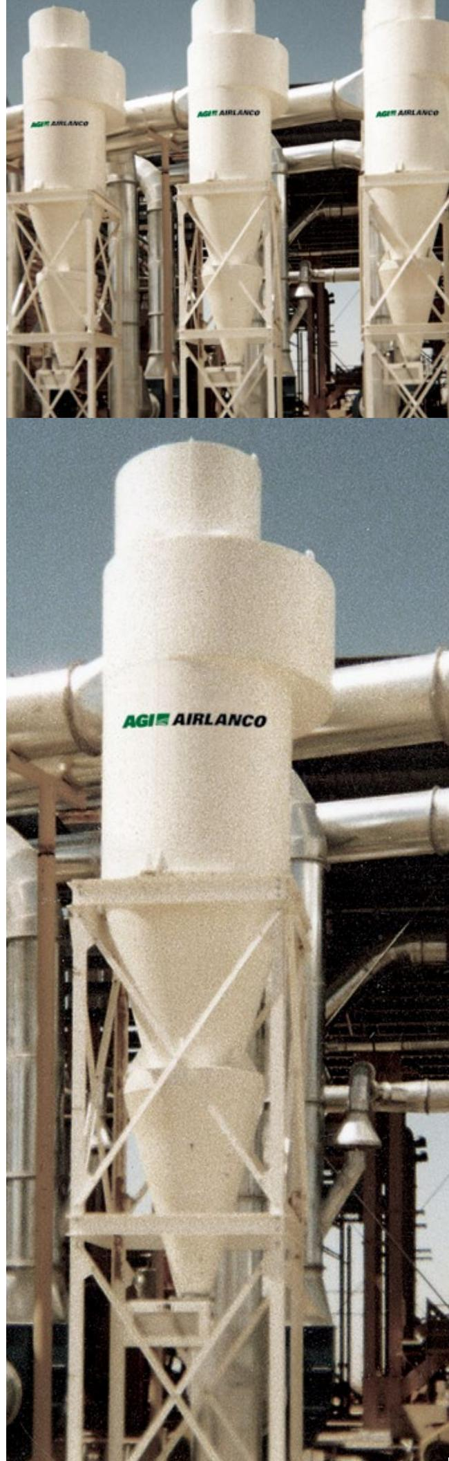
**HE SERIES CYCLONES** provide high efficiency separation of dust and particulates from plant and process air. They can withstand high temperatures, moisture content and airflow. HE Cyclones are sometimes used as pre-filters to remove large, hot or moist particles that may damage filter media in other types of collectors. Their size is limited for maximum efficiency; consequently, HE Cyclones are often ganged to meet the demands of rather large air volumes.
