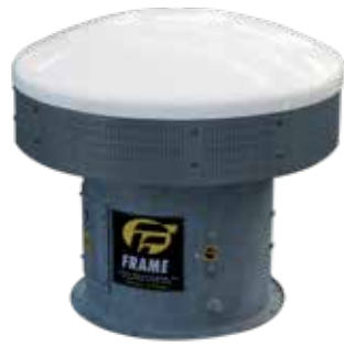
TORXEF504X2 Powered fan 0,75 kW, Volume: 8,000 m³/h @ 5mm swg – ATEX 22
