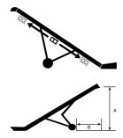
A up is conveyor discharge height (from bottom of discharge hood) at 30 degrees A down is overall conveyor height (from top of discharge hood)
