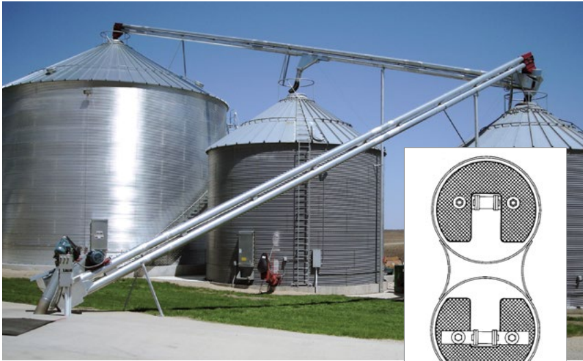
Stationary double run can be used in various applications at angles from horizontal to 60°. Lengths available in 5' increments. A flow through inlet is convenient for overhead applications.
