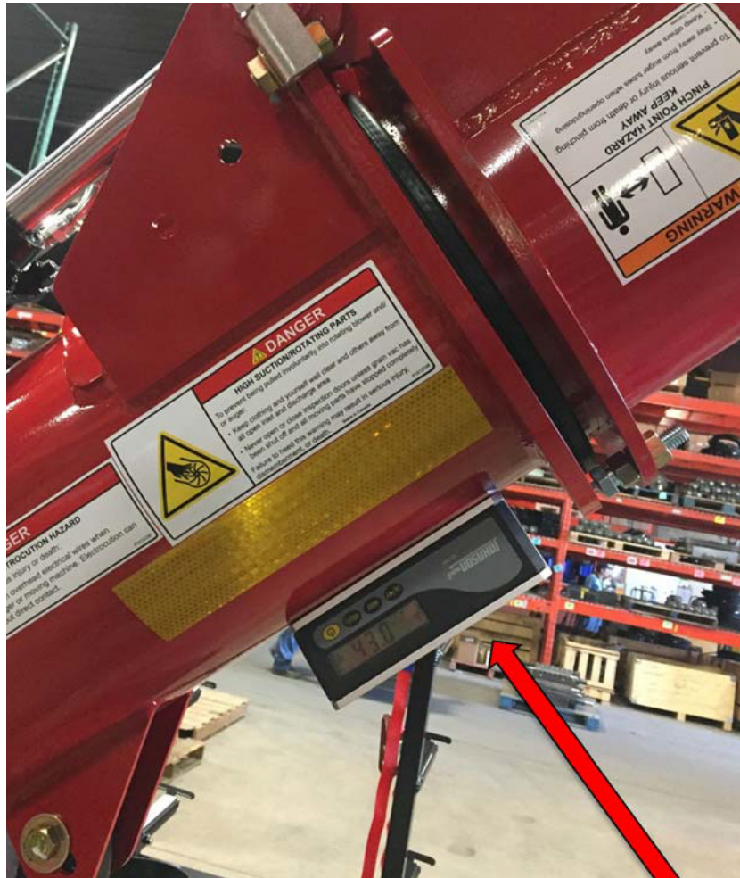
Figure 6.6 Attach Magnetic Digital Angle Finder
