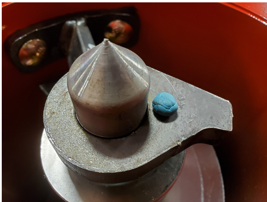
Figure 6.11 Place Putty on Middle Flyting Drive Dog
