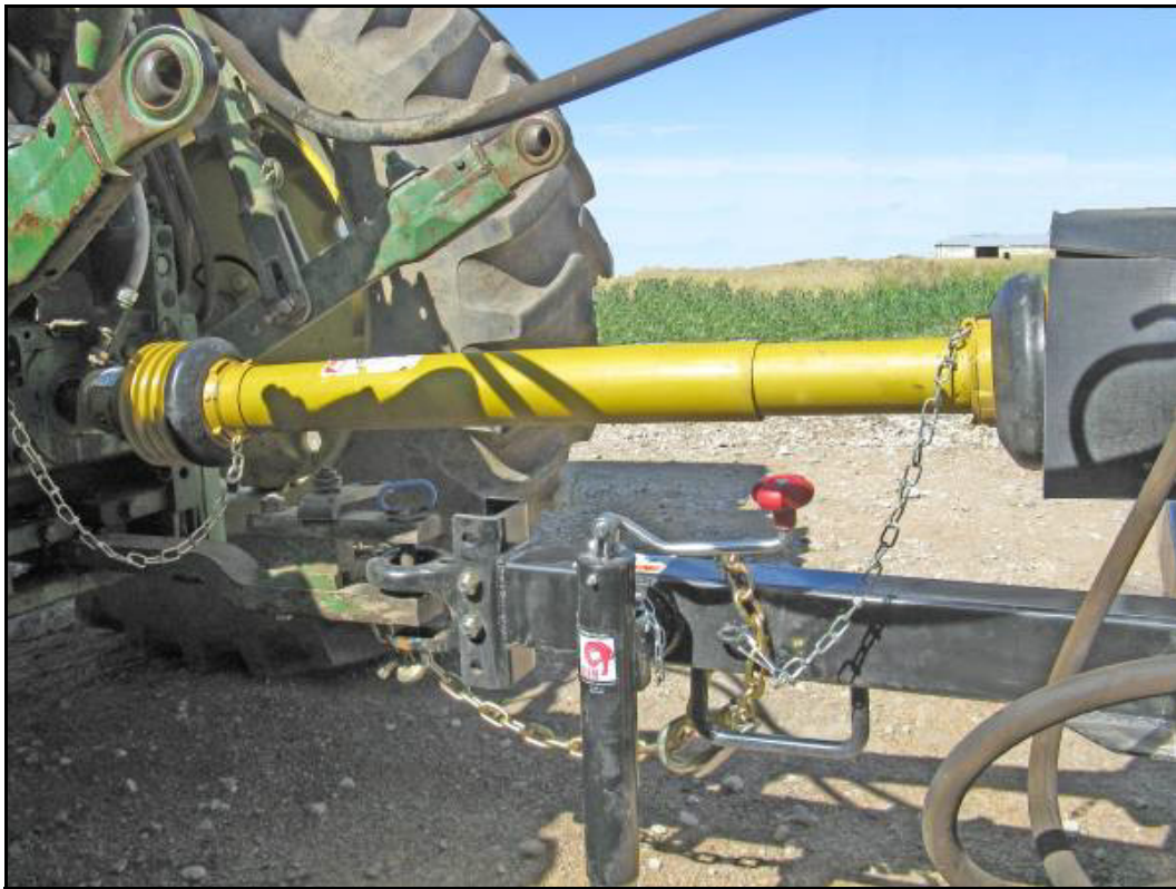
Figure 4.2 PTO Attached to Tractor
