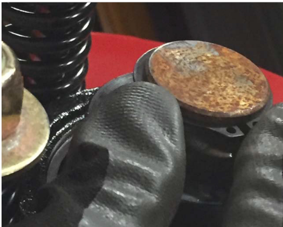
Figure 6.10 Check Snap Ring Position
