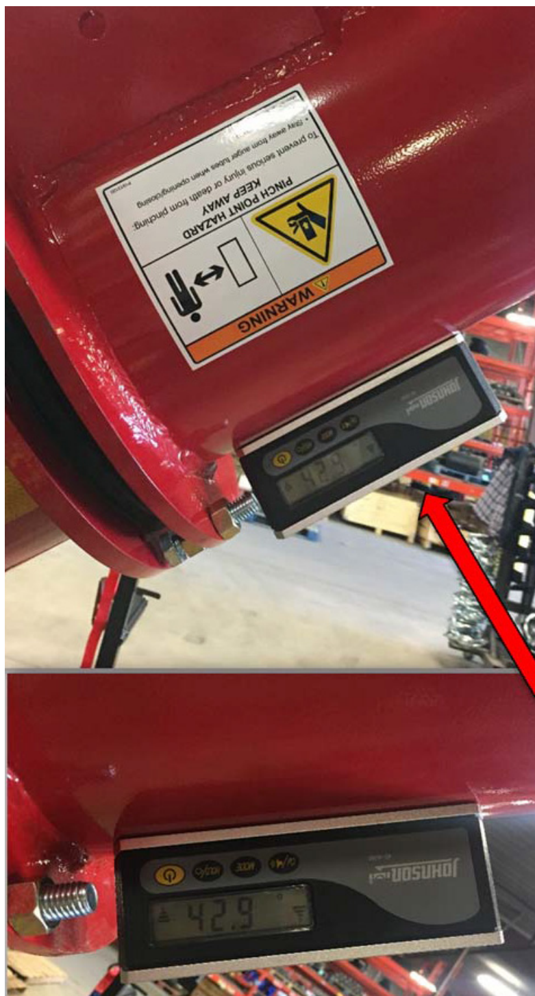
Figure 6.7 Take Middle Tube Angle Reading
