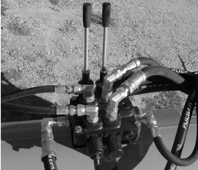
Figure 15. Power Swing Control Valve
