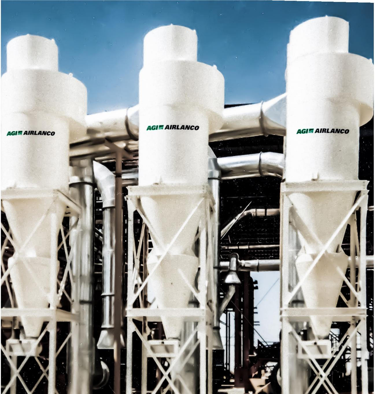
**HE Series Cyclones** provide high efficiency separation of dust and particulates from plant and process air. They can withstand high temperatures, moisture content and airflow. HE Cyclones are sometimes used as pre-filters to remove large, hot or moist particles that may damage filter media in other types of collectors. Their size is limited for maximum efficiency; consequently, HE Cyclones are often ganged to meet the demands of rather large air volumes.
