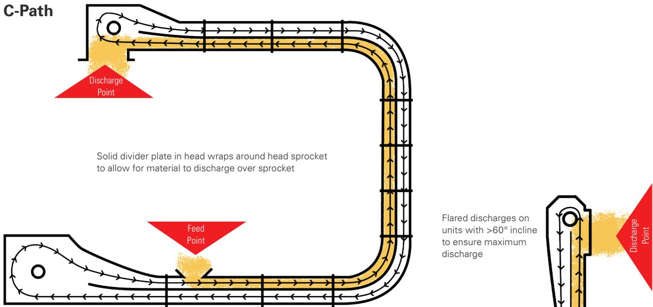
Solid divider plate in head wraps around head sprocket to allow for material to discharge over sprocket
