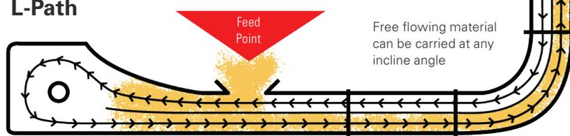
Free flowing material can be carried at any incline angle
