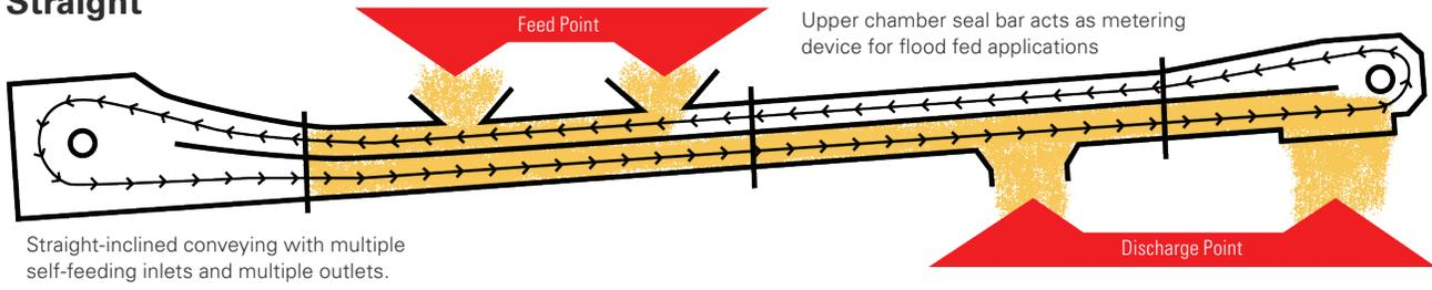
Straight-inclined conveying with multiple self-feeding inlets and multiple outlets.
