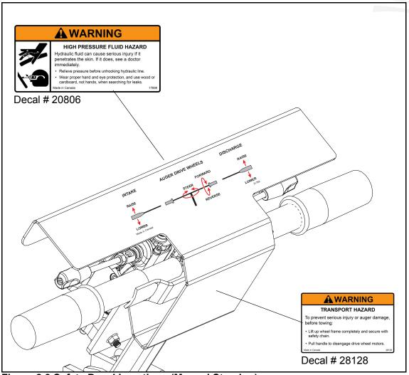
Figure 2.3 Safety Decal Locations (Manual Steering)
