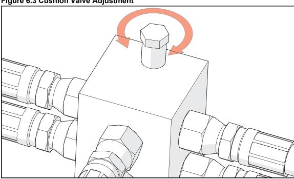
Figure 6.3 Cushion Valve Adjustment
