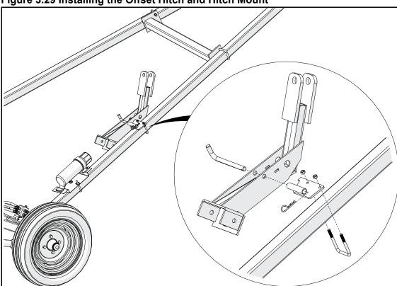
Figure 3.29 Installing the Offset Hitch and Hitch Mount
