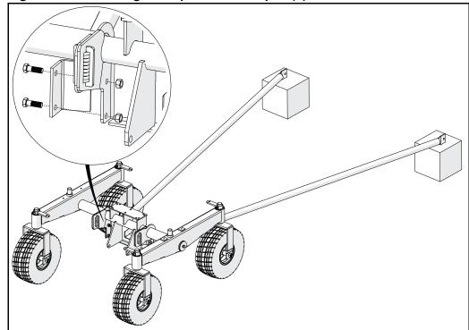
7. Attach the tabbed ends of the transport pipes to tabs on both ends of the rear axle body using a  $\frac{1}{2}$ " x 1-3/4" bolt and locknut per side (see Figure 3.12).
