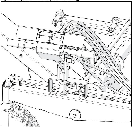
Figure 5.3 Hydraulic Controls (Hydraulic Steering) 51 Decal # 22966
