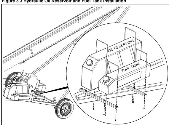
Figure 3.3 Hydraulic Oil Reservoir and Fuel Tank Installation
