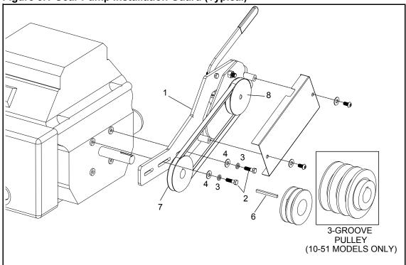
Figure 3.2 Gear Pump Installation Guard (Vanguard Engine)
