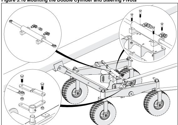
Figure 3.16 Mounting the Double Cylinder and Steering Pivots
