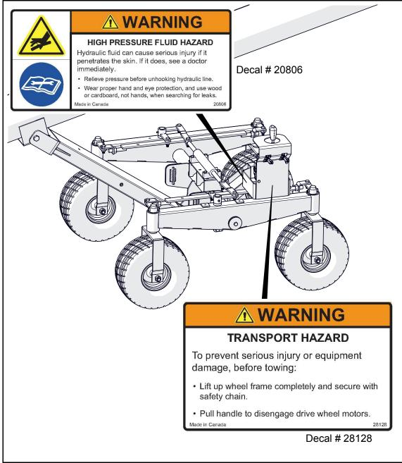
Figure 2.4 Safety Decal Locations (Hydraulic Steering)
