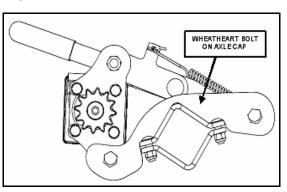
3. With the pinion gear flush with the ring gear (Figure 3.6), bolt the axle cap to the axle tube with four carriage bolts and lock-nuts.
