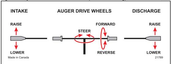
Figure 5.2 Hydraulic Controls (Manual Steering)
