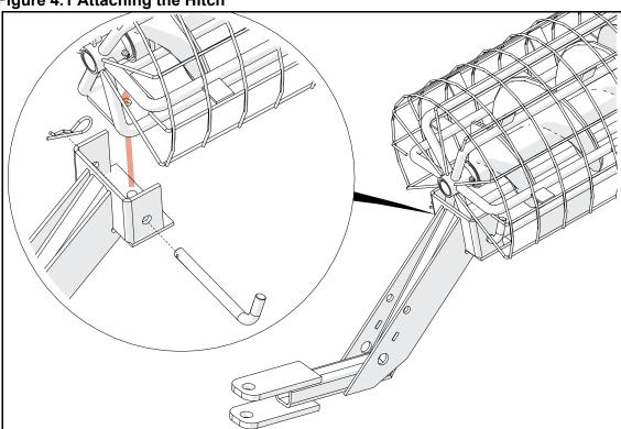
Figure 4.1 Attaching the Hitch
