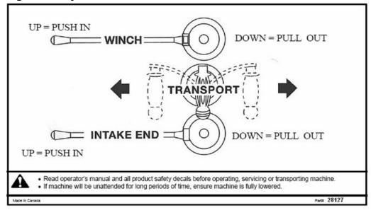
Figure 5.2 Hydraulic Control Valve
