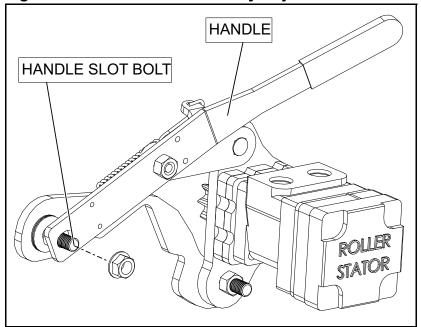
Figure 3.7 Over-Center Assembly Adjustment
