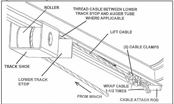
Figure 3.13 Installing the Lift Cable
