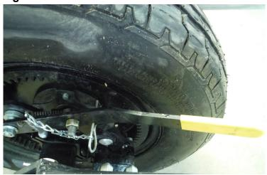
4. For transportation on public roadways, secure the v-frame to the auger frame to prevent it from accidentally slipping. Loop the snap link through the v-frame hook and attach it to the chain so there is as little slack as possible (Figure 4.3).
