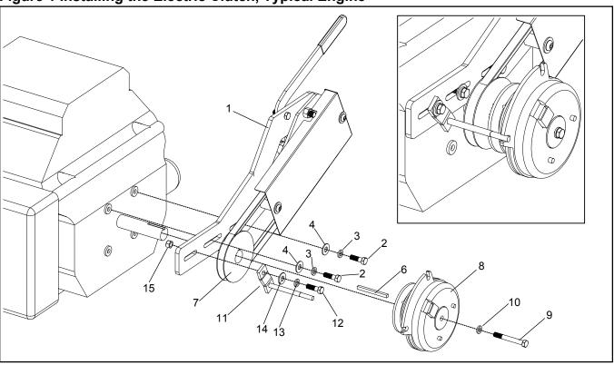
Figure 2 Installing the Electric Clutch, Vanguard Engine
