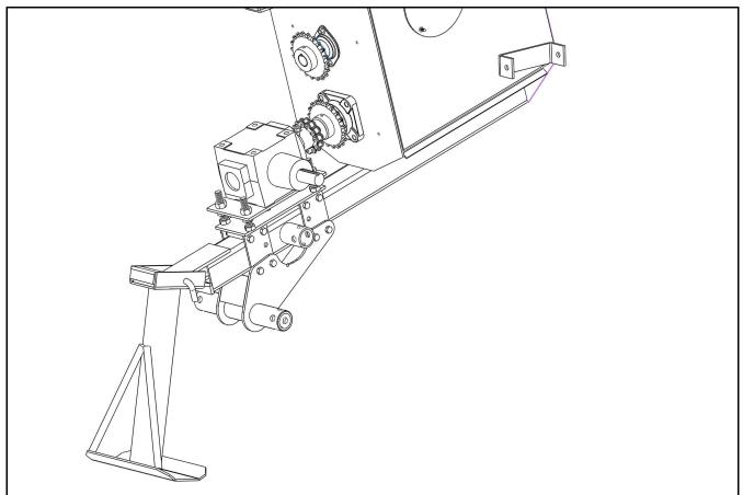
Figure 2.3 Gearbox Installed
